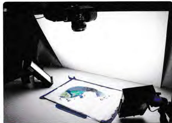
11 Bounced light makes for an even illumination over the artwork.
